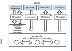
The communication architecture relies on the message bus as a broker. In addition to publish-subscribe communication, the architecture also considers request-response based communication to support integration to a variety of existing systems.
